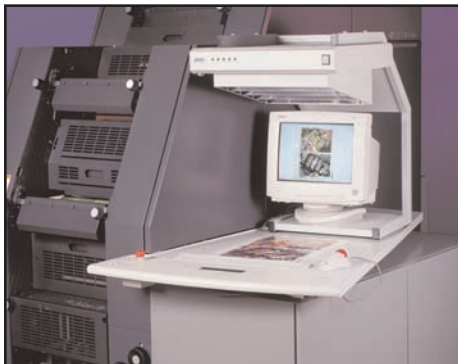
Model DIVS-1 with special reflectors to insure even illumination
