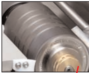
Multiple bands on the ceramic anilox roll
