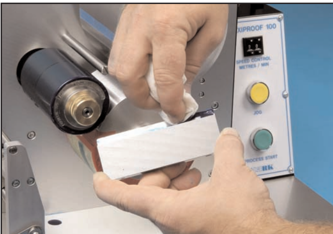
5. Clean the blade, bladeholder and side dams with a suitable solvent.
