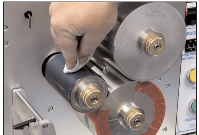
6. Clean the anilox roll while it rotates. The printing plate is also easily cleaned with the machine stopped. Use a mirror to check that it is clean.
