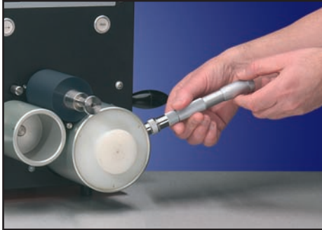
Applying ink with the IGT ink pipette
