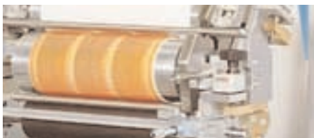
The VCM-300 flexo printing head incorporates digital read-out adjusters for the precise setting of impressions
