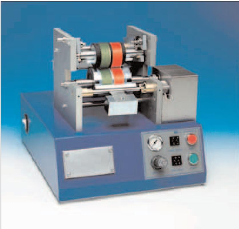
The Paste Ink Proofer is unique in featuring automated operation, eliminating the need to weigh or measure ink samples.
